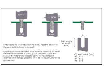
Punch or drill a hole as specified, no further hole preparation is required
