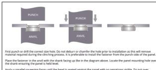
Apply a parallel squeezing force until the head is seated against the panel with no serrations visible. Do not or squeeze the fastener into the panel as this will result in panel and possibly thread deformation.
