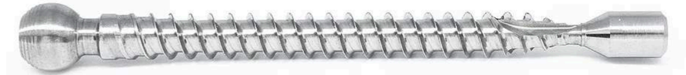
Ra: 1.16µm (before the dry electropolishing process)
