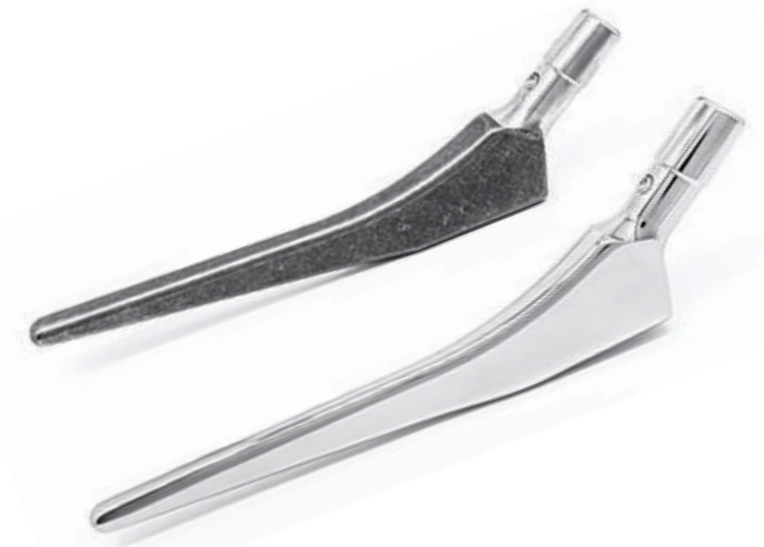
Ra: 0.09 µm (after the dry electropolishing process)
