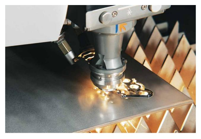
Laser cutting is an amazingly flexible technology. A wide variety of materials and thicknesses can be processed, with no limit to the shape you can obtain. Its programming is so fast that any change can be applied in any phase of your production with virtually no extra costs and time. Its precision is the highest, the quality of the cut edge is excellent and there is no part distortion.
