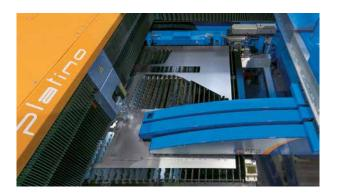
Platino equipped with LST for part sorting and stacking.
