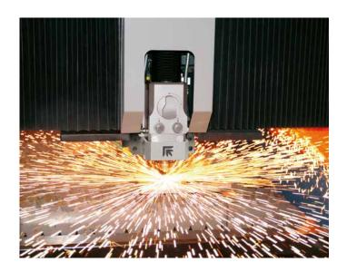
Prima Power  $CO_2$  head features safe impact protection system, process gas pipe, wide range of nozzles, F axis for controlling the focal position independently of the Z axis, lens drawer (for 5" or 7,5" lenses), capacitive sensor for automatically maintaining the preset stand-off from the sheet metal.
