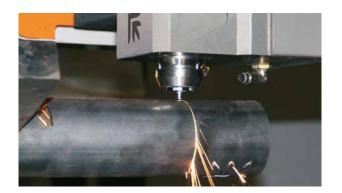
Platino easily switches to tube cutting.
