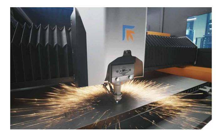
Best-in-class dynamics to grant low cycle times with excellent cutting quality. Laser Genius<sup>+</sup> can process with high quality levels a wide range of materials up to 30mm and can be equipped with laser generator with powers ranging from 2 to 10 kW.
