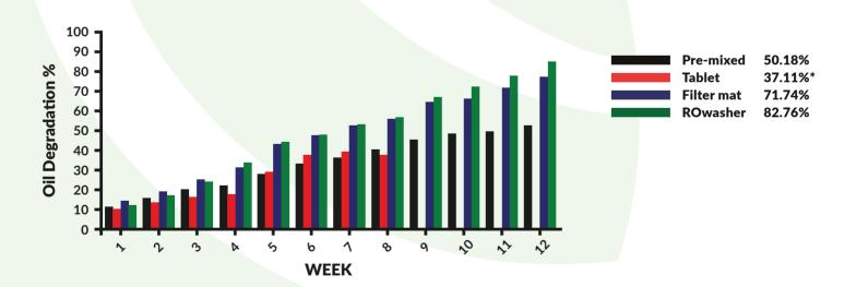
The figure shows the oil degradation rate in the ROwasher over 12 weeks compared with competitor bioremediating partswashers.
