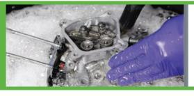
Heated to 42°C, the microbes become active in the ROwash solution and eat the oil and grease turning them into CO<sup>2</sup> and water – effectively recycling the fluid.
