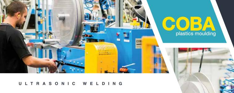
Our in-house ultrasonic welding facilities use high frequency acoustic vibrations to weld plastic components together and are a key differentiator for COBA.
