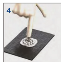
4 Firmly press the Master-Plate fastener into the adhesive until adhesive flows through the holes in the base plate.
