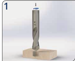
1 Prepare hole in base material to correct specification.
