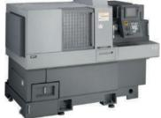
1x Polygim 32 CSL turning centre. Swiss type sliding head lathe, with 3-metre auto bar feeder and up to 32mm diameter bar capacity.
