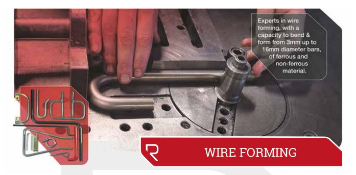
We are experts in wire forming and can bend and form 3mm - 16mm diameter bars, of ferrous and non-ferrous material. With our low tooling costs, we deliver a fast, cost-effective service.
