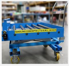
The scissor lift table with the roller top removed the need for workers to both lift and manoeuvre objects around their workplace, reducing the risk of worker fatigue and improving the efficiency of the pick and pack line.
