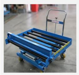
This scissor lift table solution can lift loads up to 150kg and was changed to include castor wheels, creating a piece of mobile lifting equipment. A foot pedal allows the worker to control the lift of the scissor lift table, allowing smooth operation.
