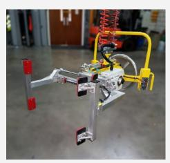
This pneumatic gripper can lift loads of up to 50kg. simple and intuitive, It grips paper core tubes, then lifts and rotates them 90 degrees so they can be placed on a mandrel as part of the manufacturing process. A pneumatic rope balancer was supplied with rotation, creating a lowthe gripper to create a full turnkey solution.
