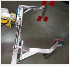
The control features are allowing workers to grip and release the product with ease. A manual handwheel is used to turn the load as the centre of mass is in line with the centre of effort rotating system.
