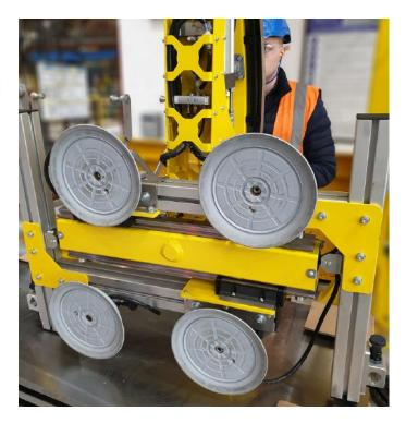
Some products are also prone to damage. To reduce the risk of this, vacuum lifting beams have padded suction feet. This is important for manufactures who do not want their products to be scratched during the production process.
