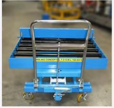
This solution was customised with a roller top. This modification made the handling of goods even easier and more efficient as it removed the need to lift goods when removing them from the scissor lift table.
