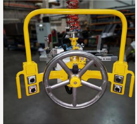
This pneumatic gripper can lift loads of up to 50kg. It grips paper core tubes, then lifts and rotates them 90 degrees so they can be placed on a mandrel as part of the manufacturing process. A pneumatic rope balancer was supplied with the gripper to create a full turnkey solution.
