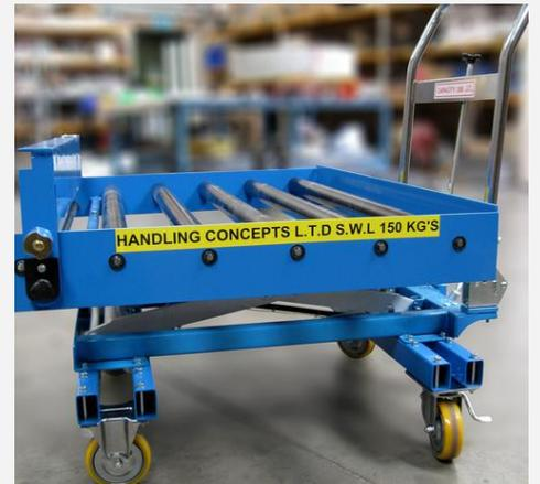
The scissor lift table with the roller top removed the need for workers to both lift and manoeuvre objects around their workplace, reducing the risk of worker fatigue and improving the efficiency of the pick and pack line.
