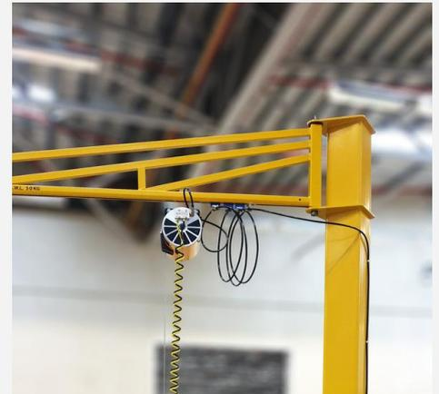
This jib crane solution can safely lift loads up to 50kg. It provides 4 metres of radial movement, allowing spare wheels to be moved between the assembly line and the warehouse. The jib crane was supplied as part of a full turnkey solution with a hoist and bespoke gripper.
