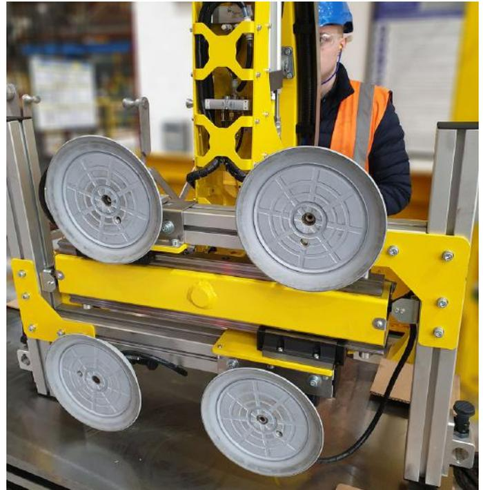
Some products are also prone to damage. To reduce the risk of this, vacuum lifting beams have padded suction feet. This is important for manufacturers who do not want their products to be scratched during the production process.
